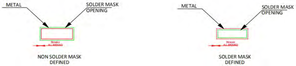
Figure 9.2 SOW8 Package Board Layout Example
