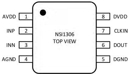
Figure 1.1 NSi1306 Package (SOP8(300mil))
