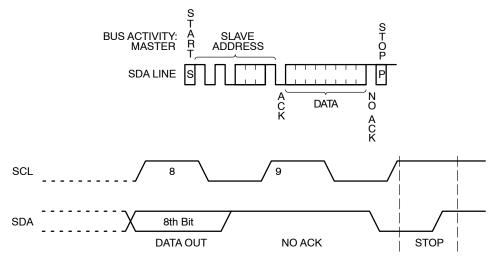
Figure 10. Immediate Address Read Timing
