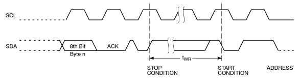
Figure 7. Write Cycle Timing
