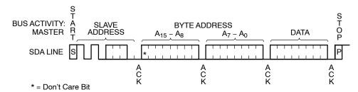
Figure 6. Byte Write Timing
