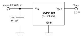
**Figure 1. Typical Application Schematics**
