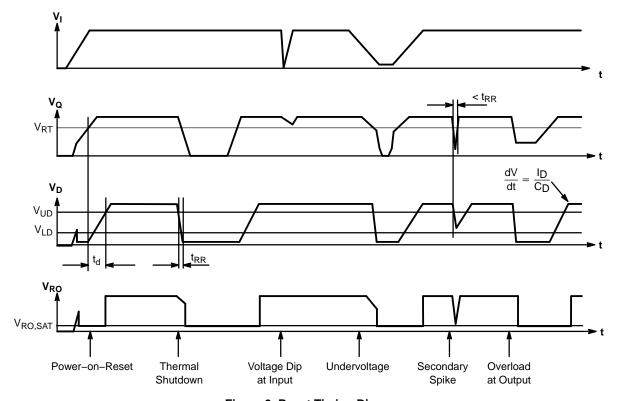
Figure 3. Reset Timing Diagram
