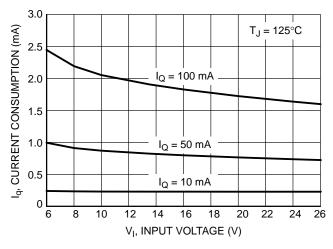
Figure 16. Quiescent Current  $I_q$  vs. Input Voltage  $V_I$
