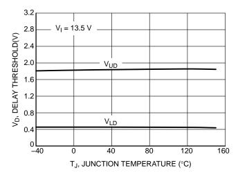
Figure 6. Switching Voltage  $\rm V_{UD}$  and  $\rm V_{LD}$  vs. Temperature  $\rm T_{J}$
