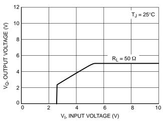
Figure 10. Output Voltage  $V_Q$  vs. Input Voltage  $V_I$
