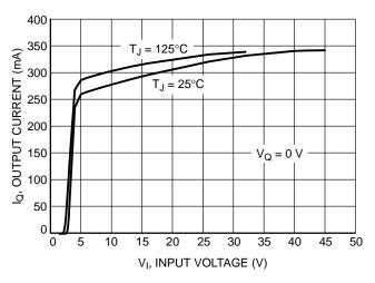
Figure 13. Output Current IQ vs. Input Voltage VI
