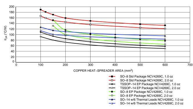
Figure 19. Junction–to–Ambient Thermal Resistance ( $\theta_{JA}$ ) vs. Heat Spreader Area
