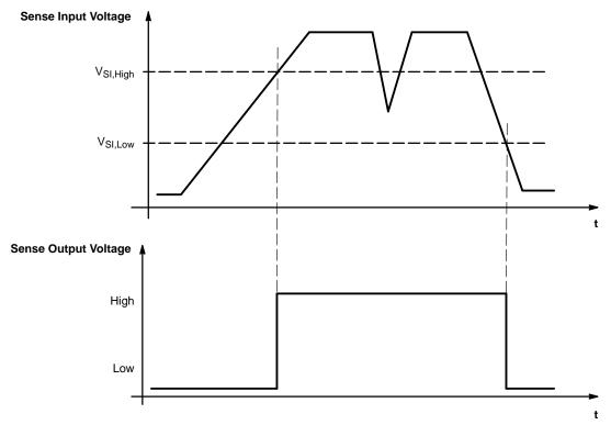
Figure 4. Sense Timing Diagram
