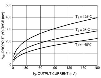
Figure 7. Drop Voltage  $V_{dr}$  vs. Output Current  $I_Q$
