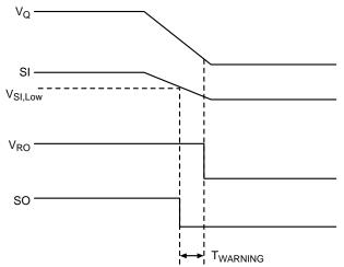
Figure 22. SO Warning Waveform Time Diagram
