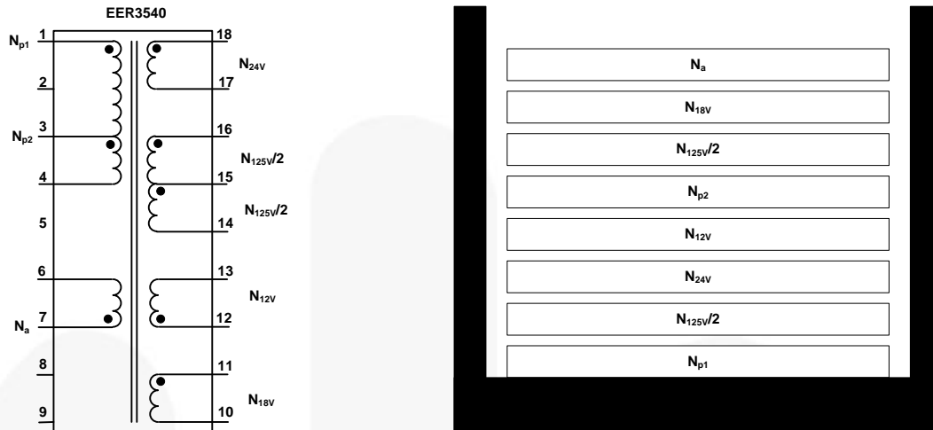
Figure 40. Transformer Schematic Diagram
