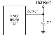
\*Includes all probe and jig capacitance
