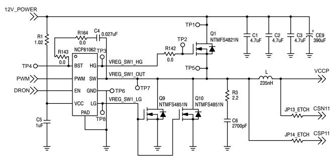
Figure 3. Application Circuit
