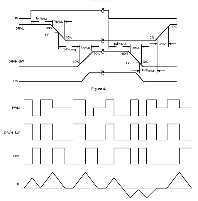
Figure 5. Timing Diagram
