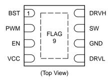
Figure 1. Pin Diagram
