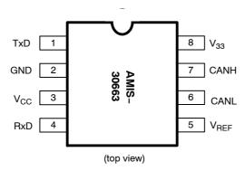
Figure 3. Pin Configuration
