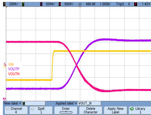
图 50. Step Response of the AMC1301 Device
